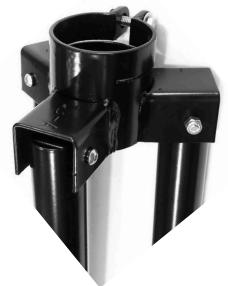
Insert screw through right side of one of the **(#1) top collar** attachment points, through the **(#5) upper leg**, and through the other side of **(#1) top collar** leg attachment point. Add **(F) nylon spacer** then **(E) lock nut**. (You will only use two nylon spacers in this portion of assembly.)
